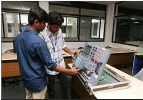
S7 1500 PLC with HMI
