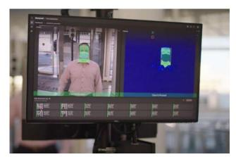
Thermal imaging camera are exploited to detect the body temperature of the person without any physical contact with him. The system can be employed in schools, colleges, malls, offices, hospitals to detect if the person has fever or not. The system assists to prevent the entry of the person with high fever inside the restricted areas to prevent the outbreak of the Covid19 which lead to pandemic situations. The sytem also prevents the spreading of various diseases.
